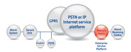
The BT Redcare Secure portfolio comprises three variants; Secure 2, Secure 3 and Secure IP – all of which protect customers with a dual path high security signalling service. Your customer will have peace of mind knowing that both of these security signalling paths are regularly monitored to comply with the latest security standards.
